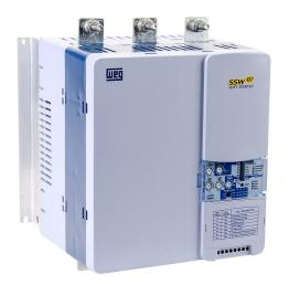
WEG Electric SSW07 series basic soft starter, 200A, 220-575 VAC at 3-phase, Trip Class 5/10/20/30, rated for 3 start/hour, internally bypassed, 3 frame. Optional Modbus RTU cards available.
