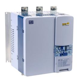
WEG Electric SSW07 series basic soft starter, 171A, 220/460/575 VAC at 3-phase, Trip Class 5/10/20/30, rated for 3 start/hour, internally bypassed. Optional Modbus RTU cards available.
