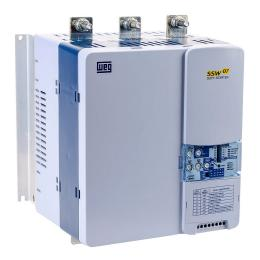
WEG Electric SSW07 series basic soft starter, 130A, 220/460/575 VAC at 3-phase, Trip Class 5/10/20/30, rated for 3 start/hour, internally bypassed. Optional Modbus RTU cards available.
