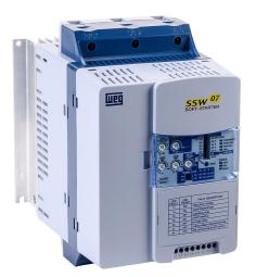
WEG Electric SSW07 series basic soft starter, 85A, 220-575 VAC at 3-phase, Trip Class 5/10/20/30, rated for 3 start/hour, internally bypassed, 2 frame. Optional Modbus RTU cards available.
