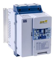
WEG Electric SSW07 series basic soft starter, 61A, 220/460/575 VAC at 3-phase, Trip Class 5/10/20/30, rated for 3 start/hour, internally bypassed. Optional Modbus RTU cards available.
