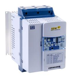
WEG Electric SSW07 series basic soft starter, 45A, 220/460/575 VAC at 3-phase, Trip Class 5/10/20/30, rated for 3 start/hour, internally bypassed. Optional Modbus RTU cards available.
