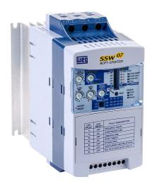
WEG Electric SSW07 series basic soft starter, 30A, 220/460/575 VAC at 3-phase, Trip Class 5/10/20/30, rated for 10 start/hour, internally bypassed. Optional Modbus RTU cards available.
