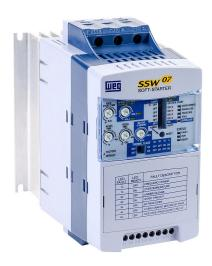
WEG Electric SSW07 series basic soft starter, 24A, 220-575 VAC at 3-phase, Trip Class 5/10/20/30, rated for 10 start/hour, internally bypassed, 1 frame. Optional Modbus RTU cards available.
