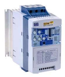
WEG Electric SSW07 series basic soft starter, 17A, 220/460/575 VAC at 3-phase, Trip Class 5/10/20/30, rated for 10 start/hour, internally bypassed. Optional Modbus RTU cards available.
