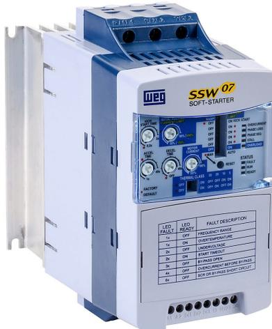
WEG Electric SSW07 series basic soft starter, 17A, 220/460/575 VAC at 3-phase, Trip Class 5/10/20/30, rated for 10 start/hour, internally bypassed. Optional Modbus RTU cards available.
