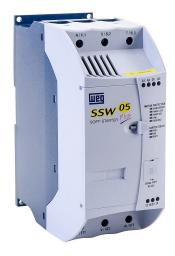
WEG Electric SSW05 series compact soft starter, 85A, 220/460 VAC at 3-phase, Trip Class 5, rated for 4 start/hour, internally bypassed.
