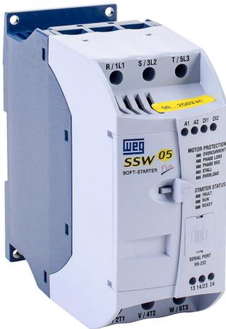
WEG Electric SSW05 series compact soft starter, 30A, 220/460 VAC at 3-phase, Trip Class 5, rated for 4 start/hour, internally bypassed.
