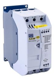
WEG Electric SSW05 series compact soft starter, 23A, 220/460 VAC at 3-phase, Trip Class 5, rated for 4 start/hour, internally bypassed.
