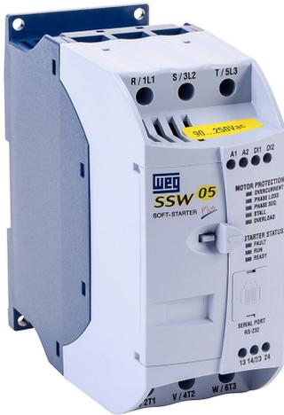
WEG Electric SSW05 series compact soft starter, 23A, 220/460 VAC at 3-phase, Trip Class 5, rated for 4 start/hour, internally bypassed.
