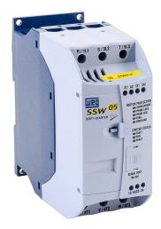
WEG Electric SSW05 series compact soft starter, 16A, 220/460 VAC at 3-phase, Trip Class 5, rated for 4 start/hour, internally bypassed.
