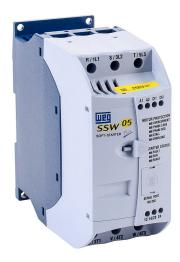
WEG Electric SSW05 series compact soft starter, 16A, 220-460 VAC at 3-phase, Trip Class 5, rated for 4 start/hour, internally bypassed, 1 frame.
