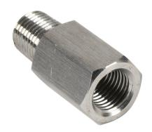
Winters heavy oil snubber, porous stainless steel element, stainless steel body, 1/4in male NPT x 1/4in female NPT.
