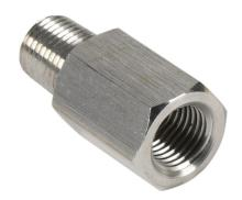
Winters air snubber, porous stainless steel element, stainless steel body, 1/4in male NPT x 1/4in female NPT.
