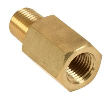
Winters heavy oil snubber, porous brass element, brass body, 1/4in male NPT x 1/4in female NPT.
