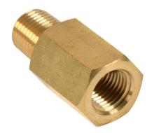
Winters air snubber, porous brass element, brass body, 1/4in male NPT x 1/4in female NPT.
