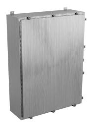
Wiegmann enclosure, NEMA 4/4X/12/13, 48 x 36 x 12in (HxWxD), wall mount, 304 stainless steel, No. 3 intermediate polished finish, single-door, (10) stainless steel clamps, padlock hasp and staple.
