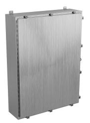
Wiegmann enclosure, NEMA 4/4X/12/13, 48 x 36 x 10in (HxWxD), wall mount, 316L stainless steel, No. 3 intermediate polished finish, single-door, (10) stainless steel clamps, padlock hasp and staple.
