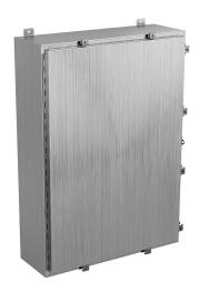
Wiegmann enclosure, NEMA 4/4X/12/13, 42 x 30 x 10in (HxWxD), wall mount, 304 stainless steel, No. 3 intermediate polished finish, single-door, (8) stainless steel clamps, padlock hasp and staple.
