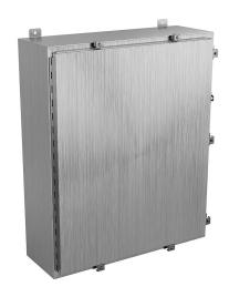
Wiegmann enclosure, NEMA 4/4X/12/13, 36 x 30 x 10in (HxWxD), wall mount, 304 stainless steel, No. 3 intermediate polished finish, single-door, (7) stainless steel clamps, padlock hasp and staple.
