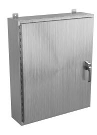
Wiegmann enclosure, NEMA 4/4X/12/13, 36 x 30 x 8in (HxWxD), wall mount, 304 stainless steel, No. 3 intermediate polished finish, single-door, 3-point 316L padlocking handle.
