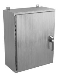
Wiegmann enclosure, NEMA 4/4X/12/13, 30 x 24 x 12in (HxWxD), wall mount, 304 stainless steel, No. 3 intermediate polished finish, single-door, 3-point 316L padlocking handle.
