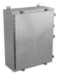
Wiegmann enclosure, NEMA 4/4X/12/13,  $30 \times 24 \times 10$  in (HxWxD), wall mount, 304 stainless steel, No. 3 intermediate polished finish, single-door, (7) stainless steel clamps, padlock hasp and staple.
