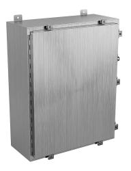
Wiegmann enclosure, NEMA 4/4X/12/13, 30 x 24 x 10in (HxWxD), wall mount, 316L stainless steel, No. 3 intermediate polished finish, single-door, (7) stainless steel clamps, padlock hasp and staple.
