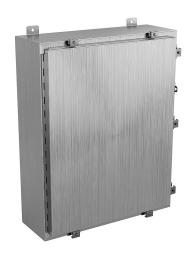
Wiegmann enclosure, NEMA 4/4X/12/13, 30 x 24 x 8in (HxWxD), wall mount, 304 stainless steel, No. 3 intermediate polished finish, single-door, (7) stainless steel clamps, padlock hasp and staple.
