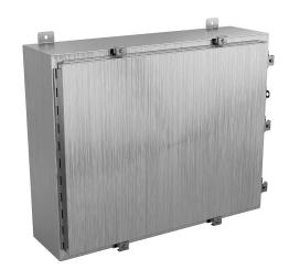
Wiegmann enclosure, NEMA 4/4X/12/13, 24 x 30 x 8in (HxWxD), wall mount, 304 stainless steel, No. 3 intermediate polished finish, single-door, (7) stainless steel clamps, padlock hasp and staple.
