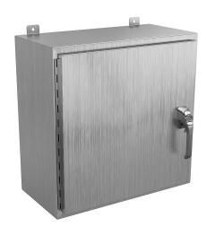
Wiegmann enclosure, NEMA 4/4X/12/13,  $24 \times 24 \times 12$ in (HxWxD), wall mount, 304 stainless steel, No. 3 intermediate polished finish, single-door, 3-point 316L padlocking handle.
