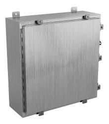
Wiegmann enclosure, NEMA 4/4X/12/13, 24 x 24 x 8in (HxWxD), wall mount, 304 stainless steel, No. 3 intermediate polished finish, single-door, (7) stainless steel clamps, padlock hasp and staple.
