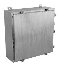
Wiegmann enclosure, NEMA 4/4X/12/13,  $24 \times 24 \times 8$ in (HxWxD), wall mount, 316L stainless steel, No. 3 intermediate polished finish, single-door, (7) stainless steel clamps, padlock hasp and staple.
