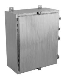
Wiegmann enclosure, NEMA 4/4X/12/13, 24 x 20 x 10in (HxWxD), wall mount, 304 stainless steel, No. 3 intermediate polished finish, single-door, (5) stainless steel clamps, padlock hasp and staple.
