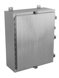
Wiegmann enclosure, NEMA 4/4X/12/13, 24 x 20 x 8in (HxWxD), wall mount, 304 stainless steel, No. 3 intermediate polished finish, single-door, (5) stainless steel clamps, padlock hasp and staple.
