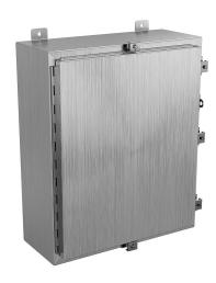
Wiegmann enclosure, NEMA 4/4X/12/13,  $24 \times 20 \times 8$ in (HxWxD), wall mount, 316L stainless steel, No. 3 intermediate polished finish, single-door, (5) stainless steel clamps, padlock hasp and staple.
