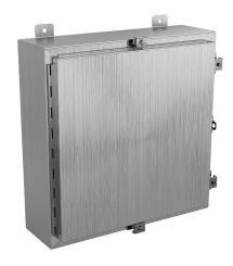
Wiegmann enclosure, NEMA 4/4X/12/13, 20 x 20 x 6in (HxWxD), wall mount, 304 stainless steel, No. 3 intermediate polished finish, single-door, (4) stainless steel clamps, padlock hasp and staple.
