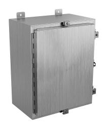
Wiegmann enclosure, NEMA 4/4X/12/13, 20 x 16 x 10in (HxWxD), wall mount, 304 stainless steel, No. 3 intermediate polished finish, single-door, (4) stainless steel clamps, padlock hasp and staple.
