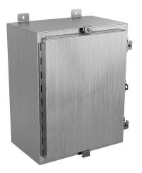
Wiegmann enclosure, NEMA 4/4X/12/13, 20 x 16 x 10in (HxWxD), wall mount, 316L stainless steel, No. 3 intermediate polished finish, single-door, (4) stainless steel clamps, padlock hasp and staple.
