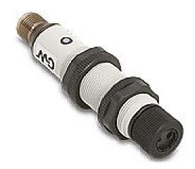
Micro Detectors fiber amplifier, tubular, 1-channel, pushbutton user interface, NPN, selectable light-on/dark-on, 10-30 VDC operating voltage, 4-pin M12 quick-disconnect.
