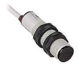
AutomationDirect photoelectric sensor, tubular, threaded, diffuse, infrared light emission, 400mm sensing distance, selectable light-on/dark-on, NPN, 250 Hz switching frequency, plastic housing, pigtail.
