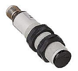
AutomationDirect photoelectric sensor, tubular, threaded, diffuse, infrared light emission, 200mm sensing distance, selectable light-on/dark-on, PNP, 250 Hz switching frequency, plastic housing, 4-pin M12 quick-disconnect.
