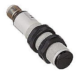
AutomationDirect photoelectric sensor, tubular, threaded, diffuse, infrared light emission, 200mm sensing distance, selectable light-on/dark-on, NPN, 250 Hz switching frequency, plastic housing, 4-pin M12 quick-disconnect.
