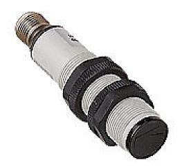
AutomationDirect photoelectric sensor, tubular, threaded, diffuse, infrared light emission, 100mm sensing distance, selectable light-on/dark-on, NPN, 250 Hz switching frequency, plastic housing, 4-pin M12 quick-disconnect.
