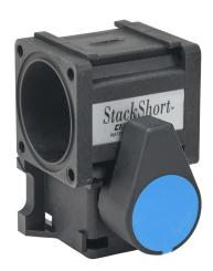
CITO StackShort modular manual valve, 2-way, 2-position, glass-filled nylon body, stackable, Cv=26.7.
