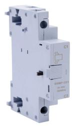
WEG Electric field installable shunt trip, right side mount, 20-24 VAC (50/60Hz) coil voltage, screw terminal. For use with MPW40 and MPW80 series manual motor protectors.
