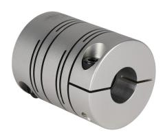
Sung-II Machinery drive coupling, servo-beam, 7075-T6 aluminum alloy, clamp, size 60, 22 x 24mm bore.
