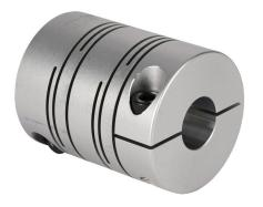
Sung-Il Machinery drive coupling, servo-beam, 7075-T6 aluminum alloy, clamp, size 60, 18 x 22mm bore.
