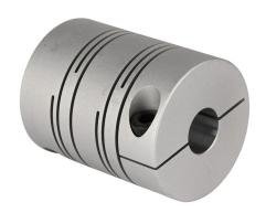
Sung-II Machinery drive coupling, servo-beam, 7075-T6 aluminum alloy, clamp, size 60, 16 x 19mm bore.
