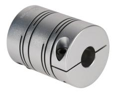
Sung-Il Machinery drive coupling, servo-beam, 7075-T6 aluminum alloy, clamp, size 49, 12 x 16mm bore.
