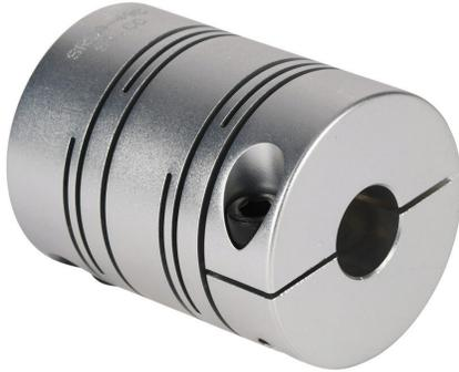
Sung-II Machinery drive coupling, servo-beam, 7075-T6 aluminum alloy, clamp, size 49, 12 x 16mm bore.
