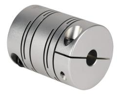
Sung-II Machinery drive coupling, servo-beam, 7075-T6 aluminum alloy, clamp, size 49, 12 x 12mm bore.
