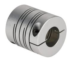
Sung-II Machinery drive coupling, servo-beam, 7075-T6 aluminum alloy, clamp, size 39, 14 x 19mm bore.
