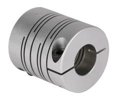
Sung-II Machinery drive coupling, servo-beam, 7075-T6 aluminum alloy, clamp, size 39, 14 x 18mm bore.
